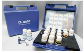
A test kit is readily available upon request. A product or combination of products contained in this kit should be effective in dewatering the majority of drilling fluid.
