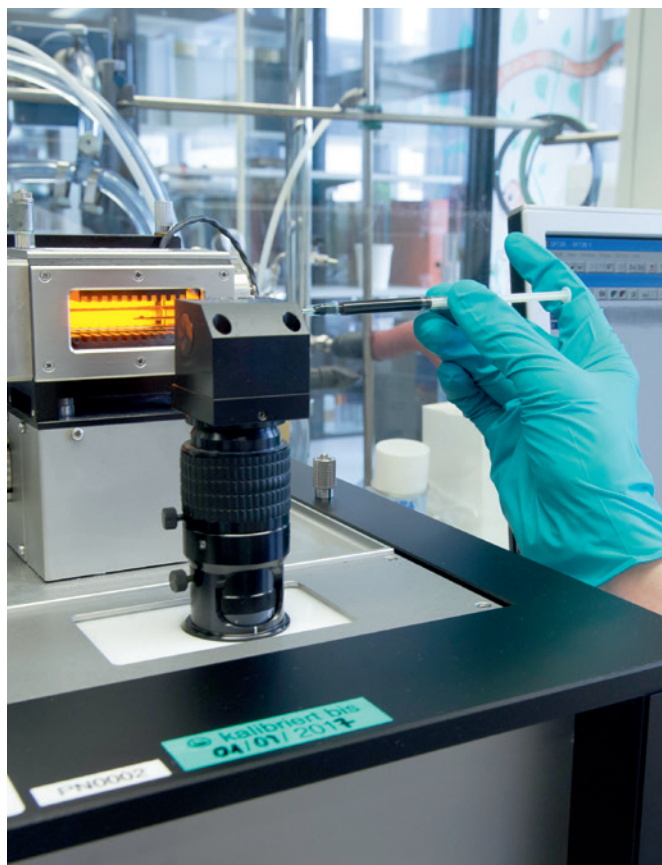
Interfacial tension measurement for formulation screening
